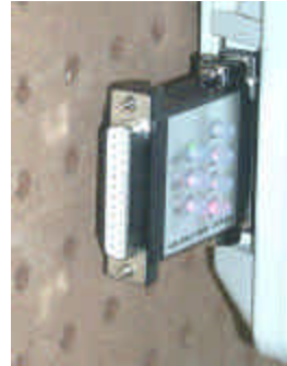
Mini-Tester inserted into SMDR Port
